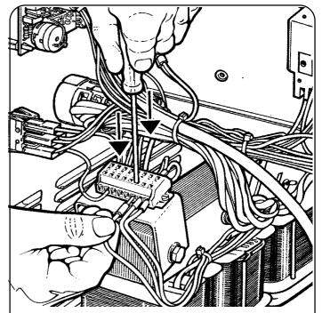
N.B. TO REACH THE VOLTAGE CHANGER REMOVE THE FIXED HOUSING (44). IMPORTANT: BEFORE CHANGING VOLTAGE MAKE SURE THAT THE MACHINE IS NO MORE CONNECTED TO THE MAINS.
